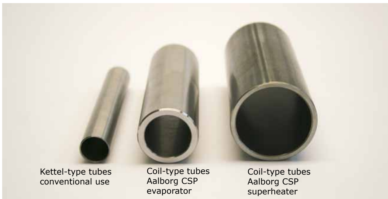
Fig. 7: Picture of the difference between the tubes used in kettle-type evaporators and the coil-type evaporator
